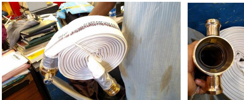
Figure 8.11: Fire Hose and Pipe
