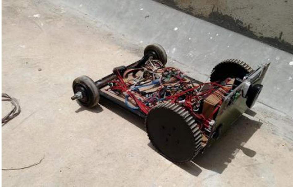
Figure 2.3: MUSAFIR v2: with improvements to Wheels and Sensors – IMU/GPS/Odometry
