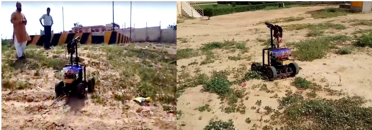
Figure 2.9: Wheeled IMR Robot with Fire hose mechanism – driving on uneven terrain
