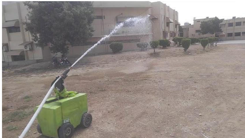
Figure 2.11: IMR Wheeled Robot with Water Hose – max distance – 35 to 45 feet forward
