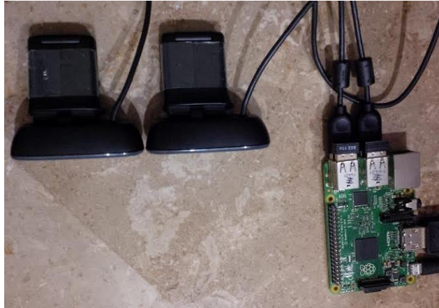
Figure 15 Stereo Vision camera with Raspberry pi
