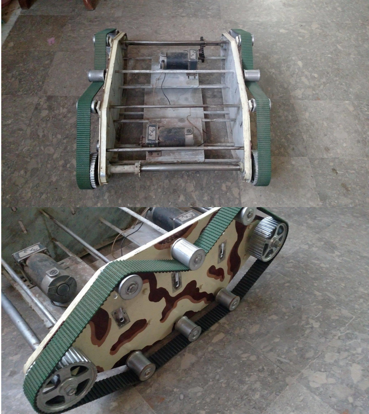
Figure 36 Actual model of tank based robot version 1.0
