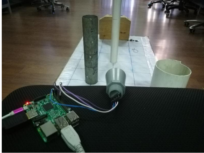
Figure 15: 4 obstacles in range of Sonar sensor
