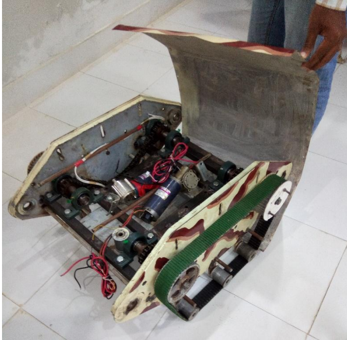
Figure 41 Actual internal design of tank based robot version 2
