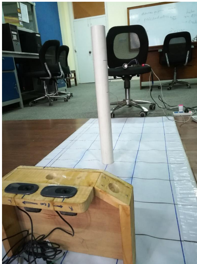
Figure 14: 2 obstacles in range of Sonar sensor
