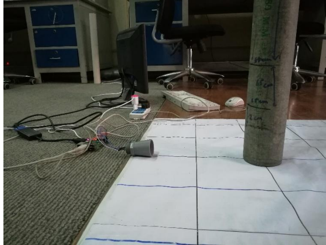
Figure 6: Steel pipe place at front at distance of 12 inch from center
